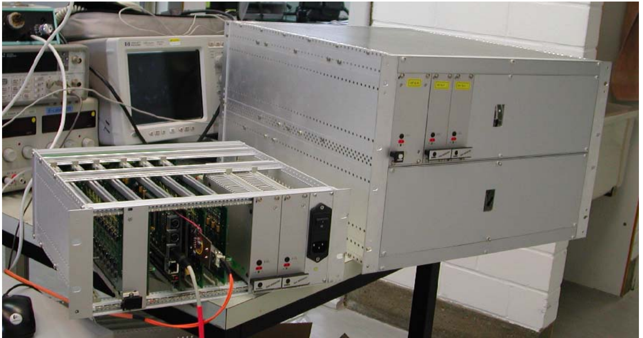
Figure 3.4.1-1 new ROE (left) versus old ROE (right)
